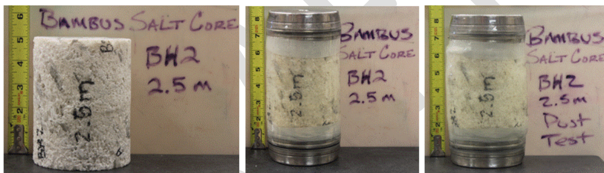
Figure 3.1. Unjacketed, jacketed pretest, and jacketed post test sample.
