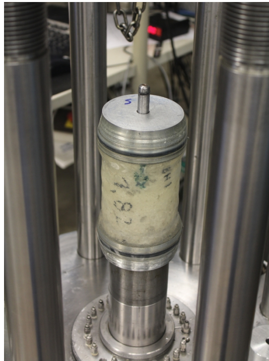
Figure 3.2. Jacketed sample with flow nipples.
